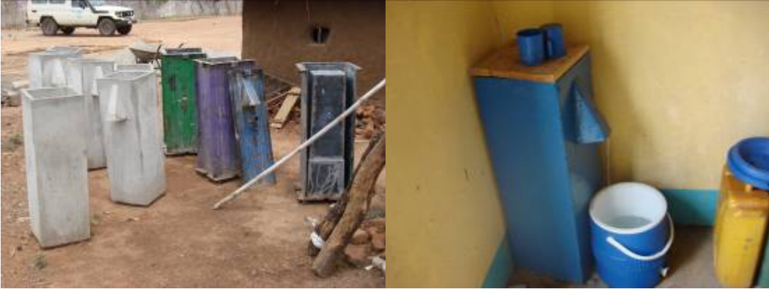
Water filter using bone-char being promoted in Jonglei State, Southern Sudan
